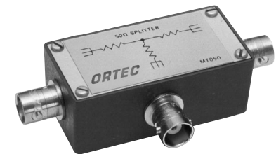
MT050 50- \Omega Matched Tee Signal Splitter One input provides two equal half-amplitude outputs and still preserves 50- \Omega termination; reflection, typically 10% (dc to over 500-MHz equivalent bandwidth); rise time, 1 ns; continuous input power, 1 W.
