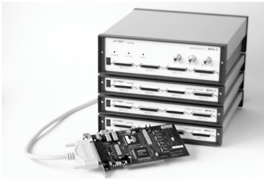
Figure 2.1: 16 port MPA-3 system
