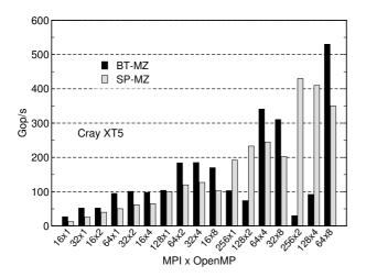
Figure 12. NPB BT-MZ and SP-MZ (class C) performance on Cray XT5 for mixed hybrid and pure MPI modes (see text for details on the mixed setup). There is no pure MPI data for 512 cores as the number of MPI processes is limited to 256 (zones) in that case.
