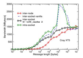
Figure 7. IMB PingPong bandwidth versus message size for inter-node, inter-socket, and intra-socket communication on an XT5. The "vanilla" variant (dashed line) uses no special options and shows pathological behavior for intermediate message sizes (see text).
