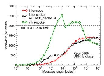
Figure 9. IMB PingPong bandwidth versus message size for inter-node, inter-socket, and intra-socket communication on a dual-socket dual-core Xeon 5160 cluster with DDR InfiniBand [4], using Intel MPI 3.1.038.
