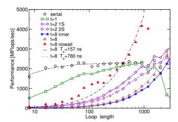
Figure 10. Impact of OpenMP loop overhead on an XT5 node for the small-N vector triad. For two cases (triangles) the model (4) was fitted to measured performance data. Note the large impact of the implied barrier (removed by the nowait clause). The stars indicate data obtained by restarting the parallel region with 8 threads on every triad loop.
