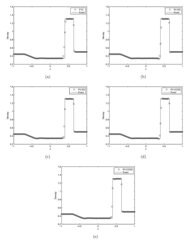
Figure 7: (a) Fourth order finite volume solution; (b) Third order DG solution; (c) Fourth order DG solution; (d) Third order DG with conservation constraints solution; (e) Fourth order DG with conservation constraints solution.
