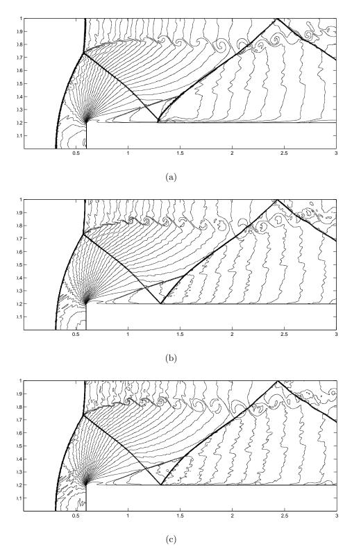
Figure 9: Forward step problem. Thirty equally spaced density contours from 0.32 to 6.15. (a) fourth order finite volume solution; (b) Fourth order DG solution; (c) Fourth order DG with conservation constraints solution.
