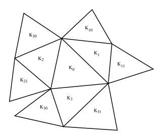
Figure 1: The stencil for preliminary construction for the finite volume scheme on cell  $\mathcal{K}_0$ .
