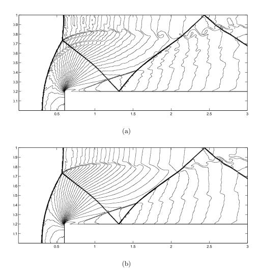
Figure 8: Forward step problem. Thirty equally spaced density contours from 0.32 to 6.15. (a) Third order DG solution; (b) Third order DG with conservation constraints solution.
