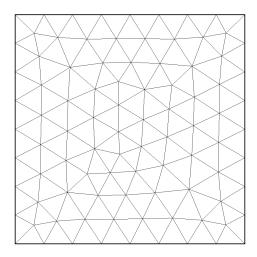
Figure 5: The typical mesh for the accuracy test for the 2D Burgers' equation and the 2D Euler equations.
