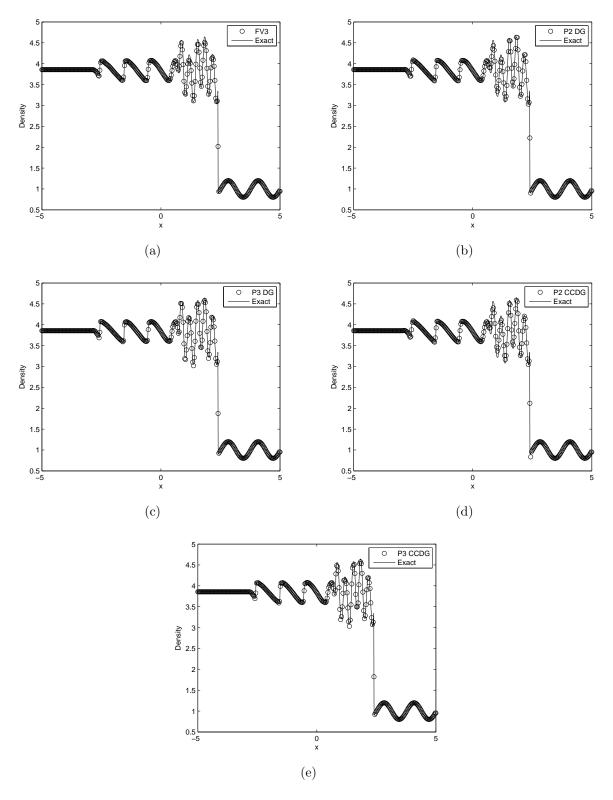
Figure 6: (a) Fourth order finite volume solution; (b) Third order DG solution; (c) Fourth order DG solution; (d) Third order DG with conservation constraints solution; (e) Fourth order DG with conservation constraints solution.
