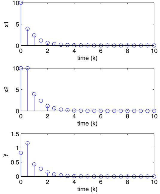
**Figure 9:** The first two panels show stability of the plant state  $x_1$  and  $x_2$ . The third panel shows the system output  $y$ .
