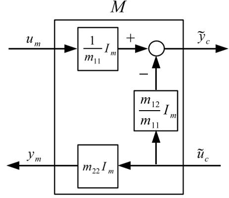
Figure 6: Implementation of  $M$  in Theorem 1
