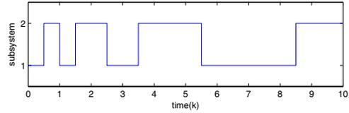
**Figure 10:** The switching signal of controller  $H_c$  that switches between subsystems 1 and 2 is shown.
