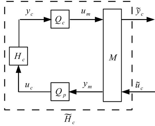
Figure 5: Proposed scheme to preserve passivity under quantization
