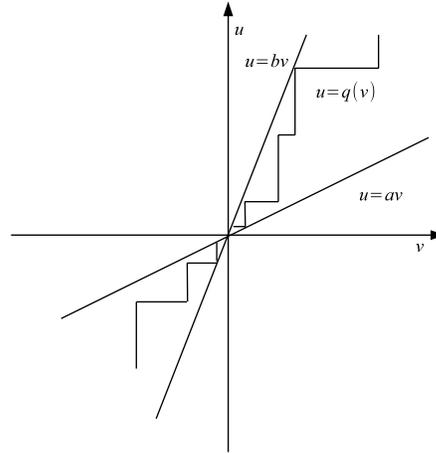
Figure 1: A general quantizer bounded by a cone
