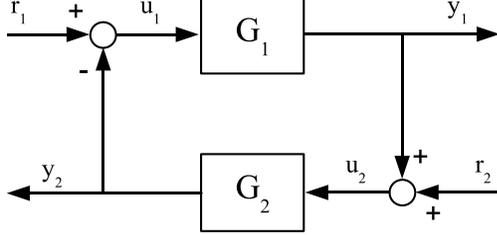
**Figure 8: The negative feedback interconnection of two systems.**
