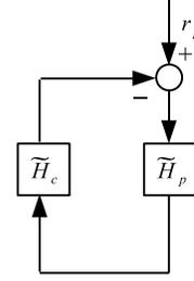
Figure 7: Negative feedback interconnection of two OSP systems
