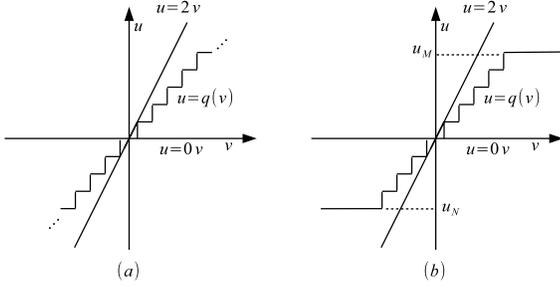
**Figure 2: (a) A uniform quantizer with infinite quantization levels (b) A uniform quantizer with finite quantization levels**
