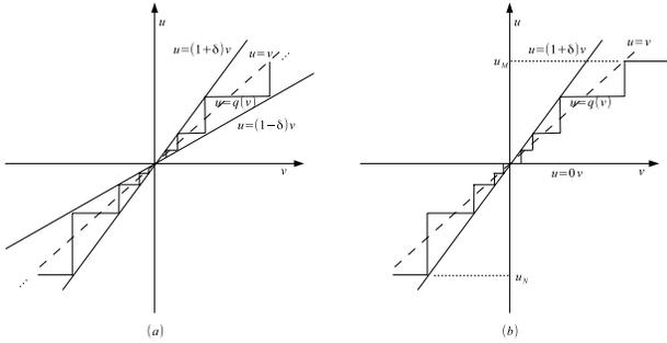
**Figure 3: (a) A logarithmic quantizer with infinite quantization levels (b) A logarithmic quantizer with finite quantization levels**
