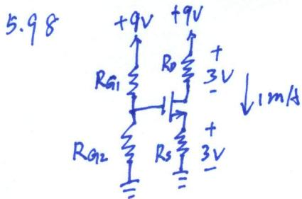
$$I_D = 1 \text{ mA} = \frac{1}{2} K_n V_{ov}^2 \Rightarrow V_{ov} = 1 \text{ V}$$
