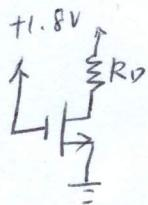
$$V_{GS} = 1.8 \text{ V}$$
