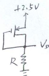
make  $i_D = 0.8 \text{ mA}$  @  $V_D = 1.5 \text{ V}$ .
