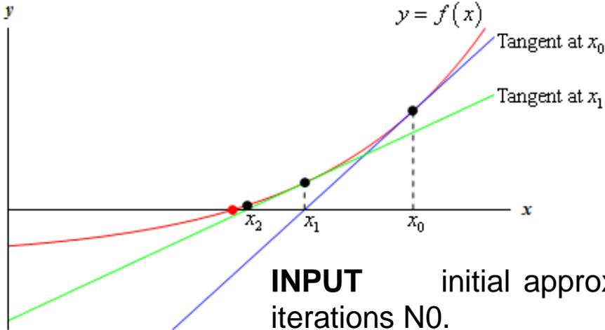
**INPUT** initial approximation  $p_0$ ; tolerance TOL; maximum number of iterations  $N_0$ .
