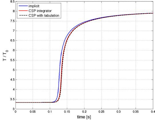
Fig. 1. Evolution of temperature (normalized by  $T_0 = 300$  K) in an igniting lean  $H_2$ -air system, using an implicit solver (blue solid line), the CSP solver (red solid line), and the CSP solver with tabulation (black dashed line). All three approaches are in good agreement, except for minor differences in the ignition time delay.
