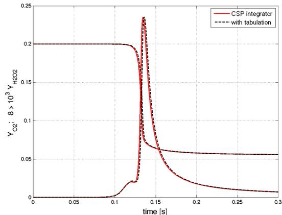
Fig. 4. Mass fractions of  $O_2$  and  $H_2O_2$  using the CSP integrator with (black dashed line) and without tabulation (red solid line). The tabulation approximation is in excellent agreement with the non-tabulated integration.
