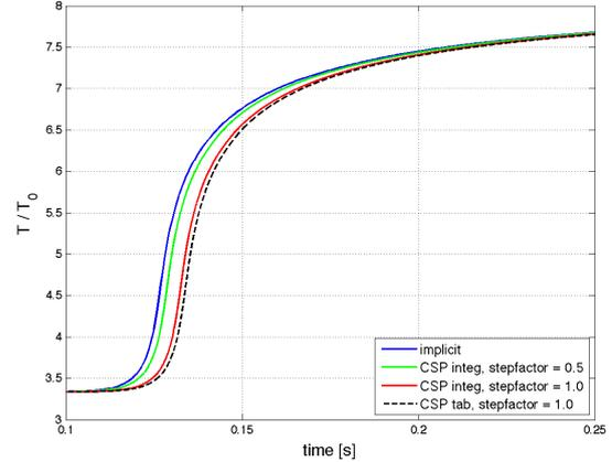
Fig. 2. Close-up of the ignition zone of Fig. 1. The CSP approximation converges to the implicit solution with decreasing time step factor  $\alpha$ :  $\Delta t = \alpha \cdot \tau_{M+1}$ .
