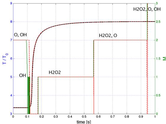
Fig. 3. Evolution of the temperature and the number of exhausted modes,  $M$ , as obtained by the CSP integrator (green) and the CSP integrator with tabulation (red). The species labels indicate the CSP radicals corresponding with the exhausted modes.
