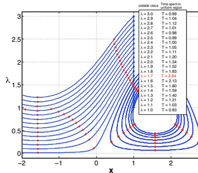
Fig. 3. Trajectories starting at  $p(0) = (1, \lambda(0))$  for a grid of  $\lambda(0)$  values. On each trajectory the zero  $\rho_h$  points are noted. The maximum averaging time is noted for each value of  $\lambda(0)$ .
