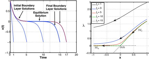
Fig. 1. Optimal solutions from GESOP<sup>©</sup> for different final times,  $t_f = 1, 5, 10, 15$  and  $17$ , where  $x(0) = 1$  and  $x(t_f) = -1$  in the time domain (left) and in the phase space (right).
