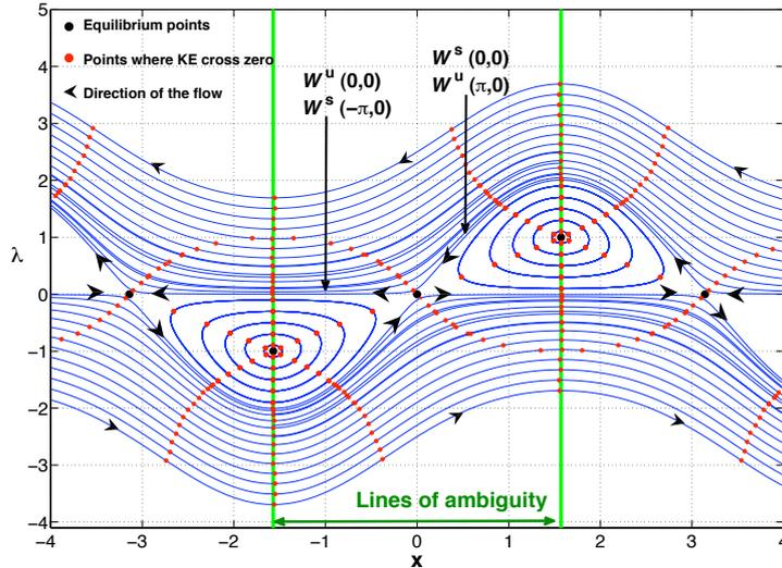
Fig. 2. Hamiltonian phase space of the system given in (3) showing stable and unstable manifolds of the equilibria, trajectories shadowing these manifolds, regions of uniformity (boundaries denoted by green circles), and lines of ambiguity.
