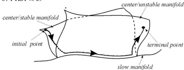
Fig. 6. Geometry of solution to partially hyper-sensitive optimal control problem in Hamiltonian phase space. Slow manifold should be 2D.
