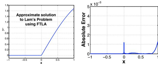
Fig. 5. **Left:** Approximation to Lam's problem using FTLA. The approximation to the stable invariant manifold is constructed with re-initializations for every  $T=0.1$ . **Right:** The absolute error between the optimal solution from GESOP and the approximate solution constructed by FTLA vs  $x$ .
