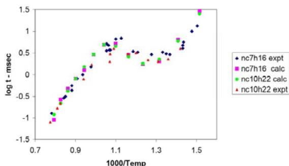
Fig. 4. Shock tube ignition delay times for n-heptane and n-decane, from experiments [18,19] and model [3].
