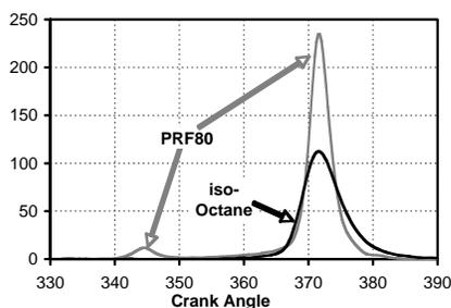
Fig. 5. Heat release rate as a function of crank angle in an HCCI engine for two fuels with different octane ratings.
