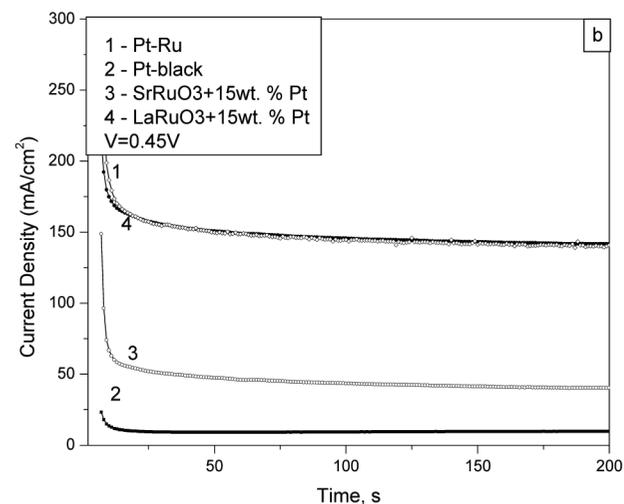
**Figure 6.** Time potential step of methanol (a) and ethanol (b) oxidation results for several catalysts (cell temperature of  $90^\circ\text{C}$ ; flow rate of  $8 \text{ mL/min}$ ).
