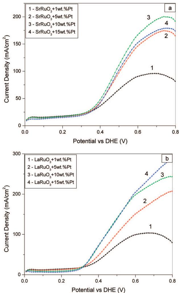
**Figure 4.** Polarization curves of ethanol oxidation by different perovskite-based catalysts: (a) SrRuO<sub>3</sub>-Pt; (b) LaRuO<sub>3</sub>-Pt. The curves are obtained in conditions such as a flow rate of 8 mL/min, potential scan rate of 20 mV/s, and 90 °C.
