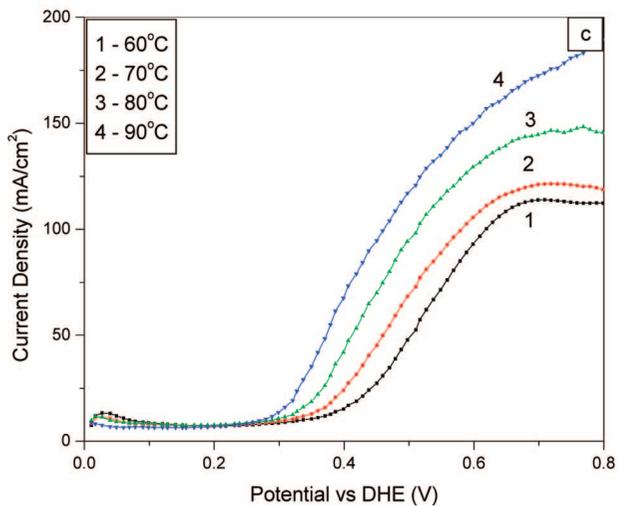
**Figure 2.** Temperature dependence of electrooxidation of ethanol by different catalysts: (a) Pt-black and Pt-Ru alloy; (b) SrRuO<sub>3</sub> + 15 wt % Pt; (c) LaRuO<sub>3</sub> + 15 wt % Pt.
