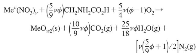
where  $\text{Me}^\nu$  is a metal with  $\nu$  = valence;  $\phi$  is a fuel to oxidizer ratio,  $\phi = 1$  means that the initial mixture does not require atmospheric oxygen for complete oxidation of fuel, while  $\phi > 1$  ( $< 1$ ) implies fuel-rich (-lean) conditions.
