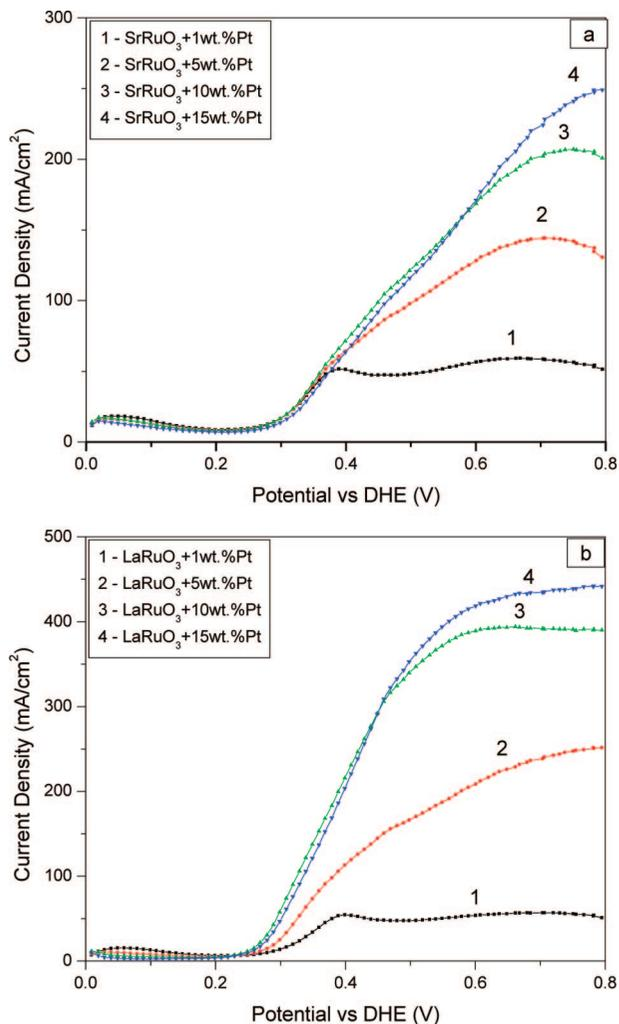
**Figure 3.** Polarization curves of methanol oxidation by different perovskite-based catalysts: (a) SrRuO<sub>3</sub>-Pt; (b) LaRuO<sub>3</sub>-Pt. The curves are obtained in conditions such as flow rate of 8 mL/min, potential scan rate of 20 mV/s, and 90 °C.
