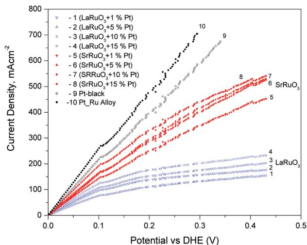
**Figure 5.** Linear scan voltammetry (LSV) results for various catalyst electrodes with hydrogen flows through anode with a flow rate of  $180 \text{ cm}^3(\text{STP}) \text{ min}^{-1}$  (all data are obtained under  $60^\circ\text{C}$  with a potential sweeping rate of  $6 \text{ mV/s}$ ).
