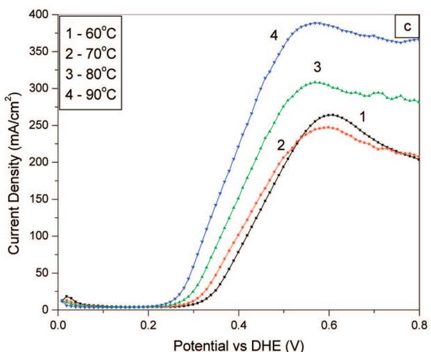
**Figure 1.** Temperature dependence of electrooxidation of methanol by different catalysts: (a) Pt-black and Pt-Ru alloy; (b) SrRuO<sub>3</sub> + 15 wt % Pt; (c) LaRuO<sub>3</sub> + 15 wt % Pt.
