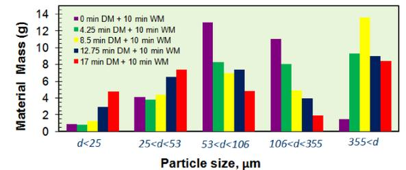
Fig. 5. Material yield of ball milled Ni/Al materials.
