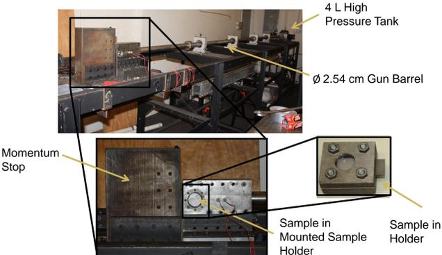
Fig. 3. Gas gun and experimental configuration for impact ignition experiments.
