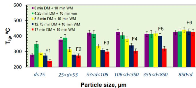
Fig. 9. Ignition temperature for Ni/Al materials obtained at various milling conditions as a function of particle size.
