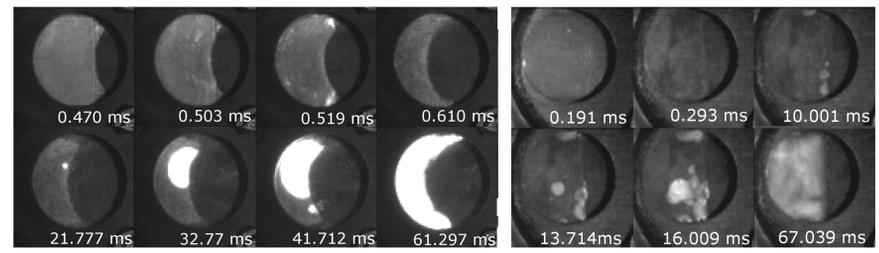
Fig. 7. Impact ignition test of Ni/Al dry milled for 12.75 min and wet milled for 10 min with a plunger of 0.4" radius at 130m/s.
