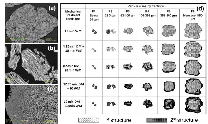
Fig. 6. Ni/Al particles with only 1<sup>st</sup> structure (a), only 2<sup>nd</sup> structure (b), combination of both structures (c), and diagram (d) showing all possible combinations.
