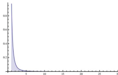
Since  $\int_1^\infty \frac{1}{x} dx$  diverges, the area under the curve  $y = 1/x$  on the interval  $[1, \infty)$  (shown on the left above) is not finite.
