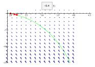
▶ We can write down algebraic formulas for the endpoint of this arrow  $(x_1, y_1)$ . We know that  $x_1 = x_0 + h$ . We have the slope of the arrow is  $F(x_0, y_0) = \frac{y_1 - y_0}{x_1 - x_0} = \frac{y_1 - y_0}{h}$ .
