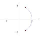
We can solve the equation for x to get the function  $x = \sqrt{4 - y^2}$  (taking the positive square root because x is positive on the portion we are interested in).
