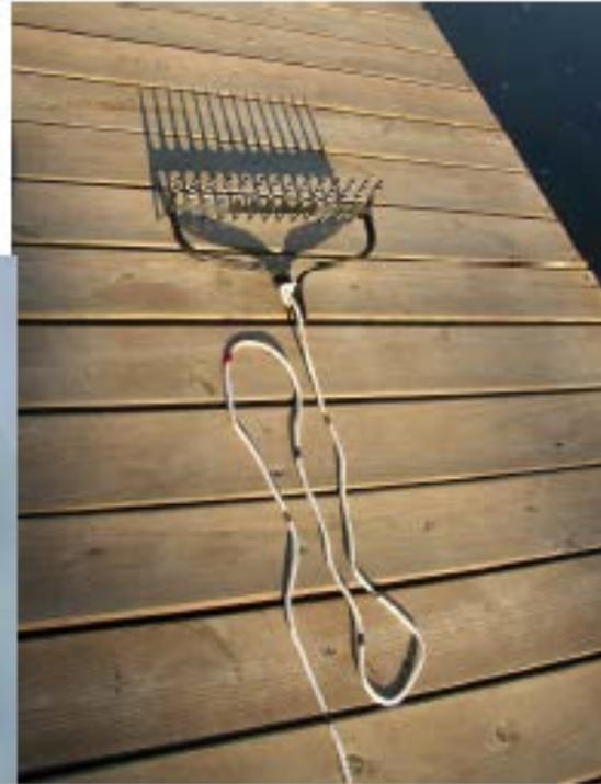
**Figure 1: Double-headed rake for aquatic vegetation sampling**
