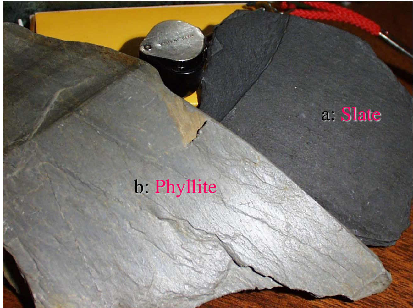
Figure 22.1. Examples of foliated metamorphic rocks. a. Slate. b. Phyllite. Note the difference in reflectance on the foliation surfaces between a and b: phyllite is characterized by a satiny sheen. Winter (2001) An Introduction to Igneous and Metamorphic Petrology . Prentice Hall.
