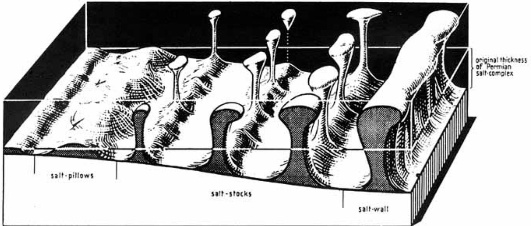
**Figure 4.33.** Block diagram of subsurface **salt diapirs** in Northern Germany. After Trusheim (1960), *Bull. Amer. Assoc. Petrol. Geol.*, **44**, 1519-1540 © AAPG.
