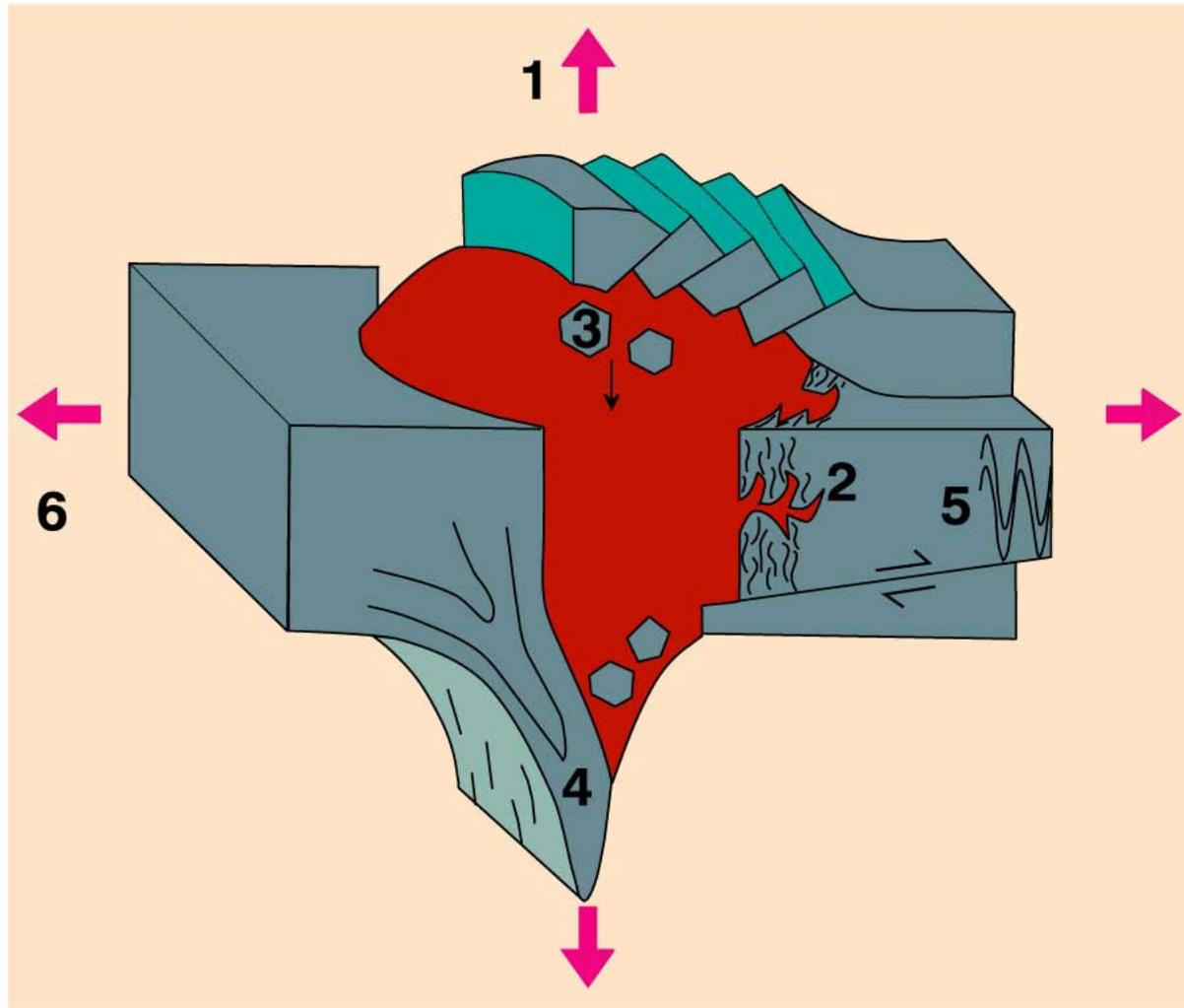
**Figure 4.34.** Diagrammatic illustration of proposed **pluton emplacement mechanisms**. **1- doming** of roof; **2- wall rock assimilation**, partial melting, zone melting; **3- stoping**; **4- ductile wall rock deformation** and wall rock **return flow**; **5- lateral wall rock displacement** by faulting or folding; **6- (and 1)- emplacement into extensional environment**. After Paterson *et al.* (1991), *Contact Metamorphism. Rev. in Mineralogy*, **26**, pp. 105-206. © Min. Soc. Amer.
