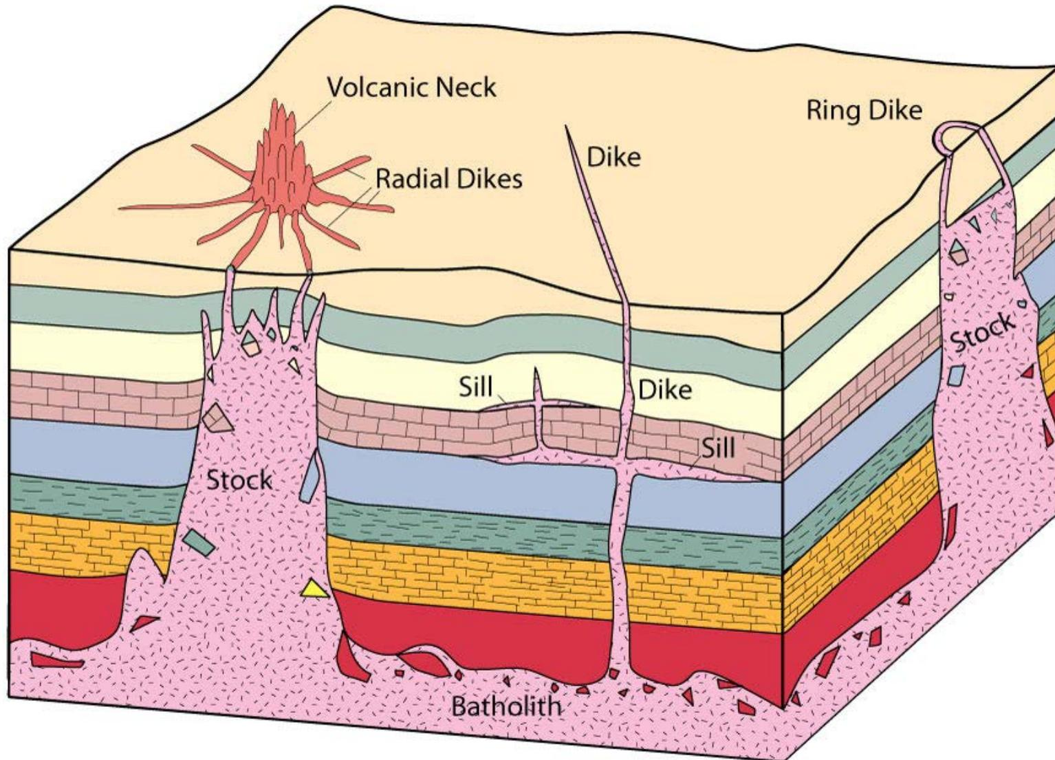
**Figure 4.20.** Schematic block diagram of some intrusive bodies.
