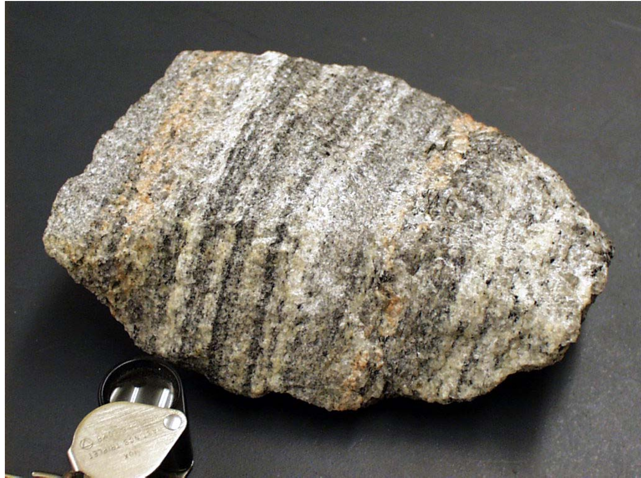
Figure 22.1d. Quartzo-feldspathic gneiss with obvious layering. Winter (2001) An Introduction to Igneous and Metamorphic Petrology . Prentice Hall.
