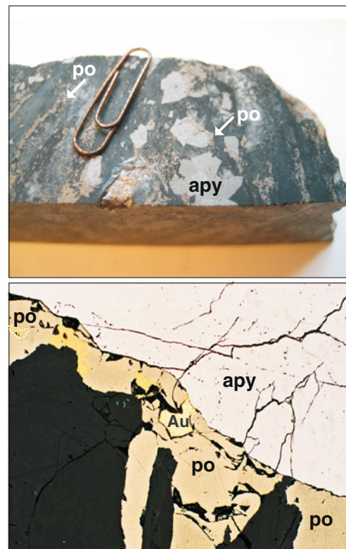
Fig. 4 a Photograph of sample HM020, showing pyrrhotite ( po ) surrounding arsenopyrite ( apy ) crystals and exhibiting parallelism to the foliation ( S ). b Photomicrograph of sample HM020 (field of view = 0.64 mm)
