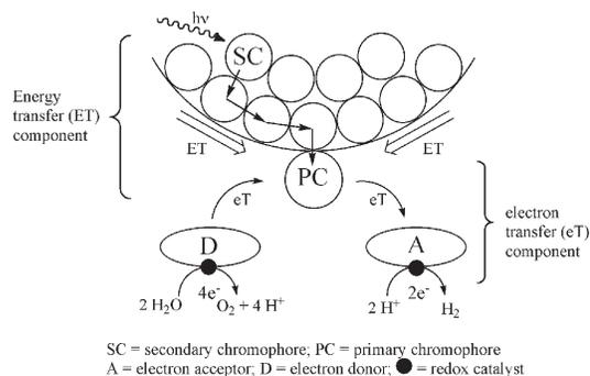
**Figure 1.** Energy transfer (ET) and electron transfer (eT) components of an artificial photosynthetic system (APS): Energy transfer from the secondary chromophores to the primary chromophore leads to electron transfer and the production of H<sub>2</sub> by way of a redox catalyst.
