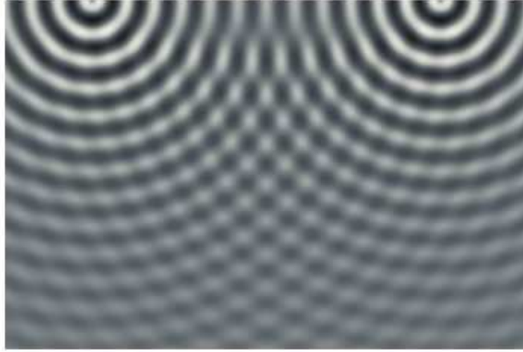
FIGURE 1.1. Interference of waves emitted from two slits
