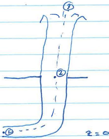
$$P_1 + \frac{1}{2} \rho v_1^2 + \rho g z_1 = P_2 + \frac{1}{2} \rho v_2^2 + \rho g z_2 = P_3 + \frac{1}{2} \rho v_3^2 + \rho g z_3$$
