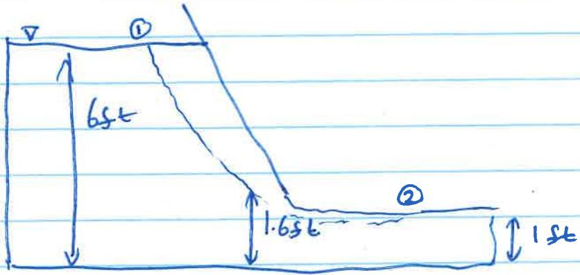
$$q_1 + \frac{1}{2} \gamma v_1^2 + \gamma g z_1 = q_2 + \frac{1}{2} \gamma v_2^2 + \gamma g z_2$$
