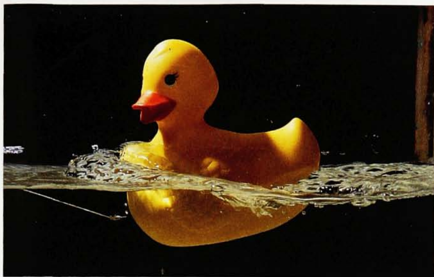
FIGURE 1. RUBBER DUCKY being towed in a flow tank just under (left) and just over (bottom) its hull speed. Notice that at the higher speed this small surface ship tips upward and its stern wave disappears.
