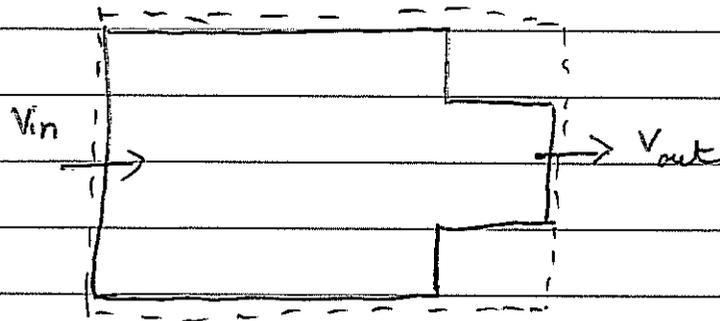
$$(i) \quad v_{in} A_{in} = v_{out} A_{out}$$
