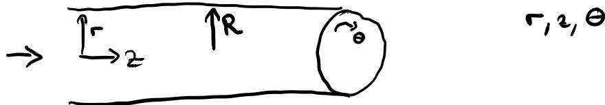
$$\text{Continuity} \Rightarrow \frac{\delta g}{\delta t} + \frac{1}{r} \left( \frac{\delta}{\delta r} (r g v_r) \right) + \frac{1}{r} \frac{\delta (g v_\theta)}{\delta \theta} + \frac{\delta (g v_z)}{\delta z} = 0$$
