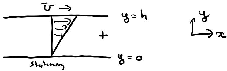
$$\textcircled{1} \text{ Incompressible } \Rightarrow \frac{\partial u}{\partial x} + \frac{\partial v}{\partial y} + \frac{\partial w}{\partial z} = 0$$
