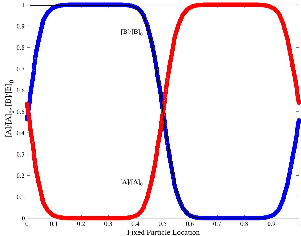
**Figure 3.** Diffusion on a periodic 1- $d$  domain via probabilistic mass transfer among 10,000 fixed particles in space. Total time = 100 and  $D=10^{-5}$ . Each particle has A (red) and B (blue) mass, with initial condition on each particle  $A(0.5 \leq x \leq 1)=B(0 \leq x \leq 0.5)=1$  and zero otherwise. Black line is the analytic solution for the B diffusion profile in the center of the domain.
