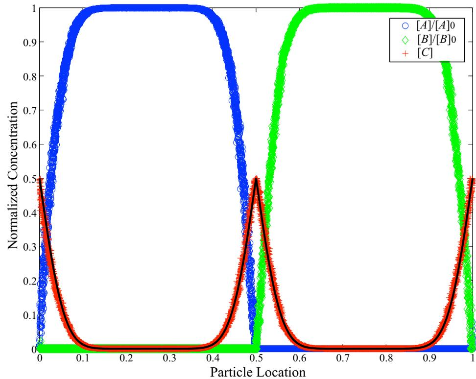
**Figure 7.** Single realization of fast (essentially instantaneous) reaction resulting from initially sharp interface between A and B. Periodic domain had initial interfaces at  $x=0=1$  and  $x=0.5$ . Diffusion is simulated half by random walks and half by mass transfer among stationary particles between motions. Black line is analytic solution.
