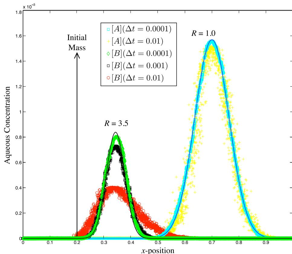
**Figure 8.** Mobile concentrations (symbols) from simulations of particles carrying species A and B that interact with immobile particles. Distribution coefficients are  $K_d^A=0$  and  $K_d^B=2.5$  for retardation coefficients of 1 and 3.5, respectively. Time step sizes from 0.01 to 0.0001 are shown. Analytic solutions shown by continuous curves.
