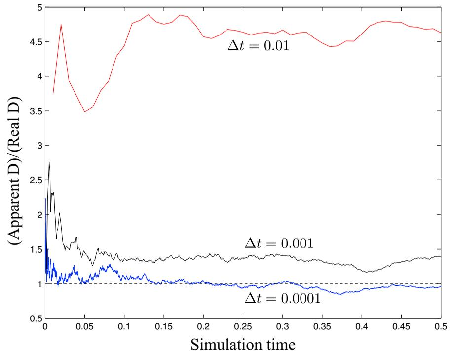
**Figure 9.** Ratio of simulated to analytic plume variance for the  $R = 3.5$  plumes for timestep sizes (top) 0.01, (middle) 0.001, and (bottom) 0.0001.
