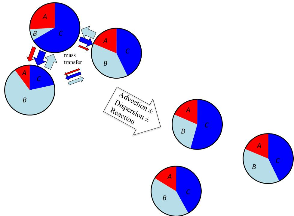
**Figure 1.** Schematic representation of mass transfer and particle motion operations split in a time step. The mass transfer is proportional to mass difference between particles and the probability of colocation, which decreases with separation distance. Colored arrow size is representative of transfers according to equation (7).
