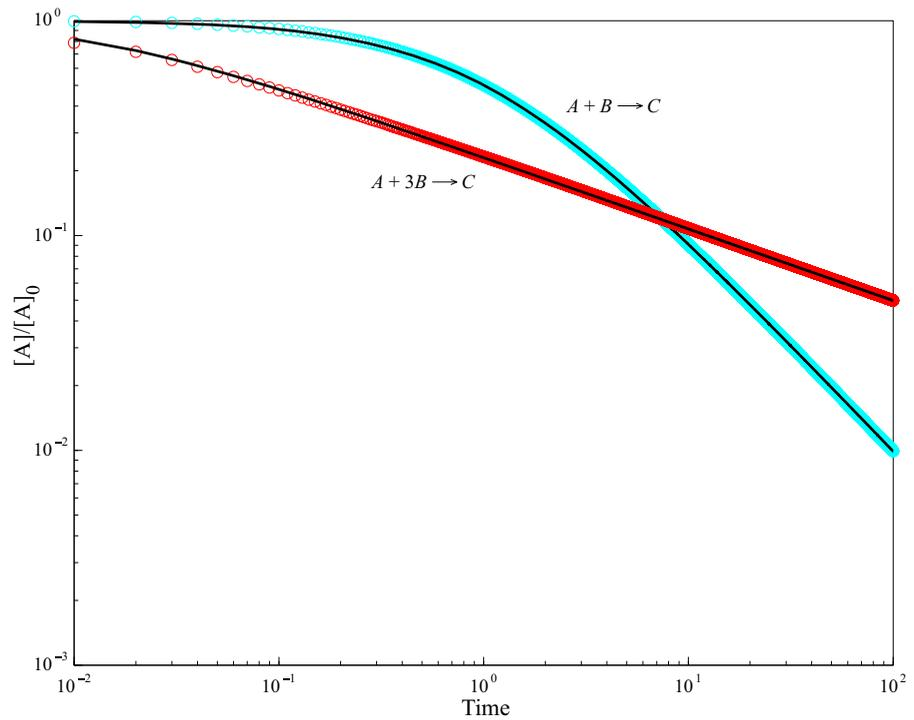
**Figure 4.** Simulated domain-average  $[A](t)/[A]_0$  due to diffusive mass transfer of  $A$  and  $B$  and reaction according to (1) on a periodic  $1-d$  domain among 1,000 fixed particles in space. Total time = 100,  $D=10^{-2}$ ,  $k_f = 1$ ,  $[A]_0 = 1$ , and  $[B]_0 = q[A]_0$ . Simulations are for  $p=1$  and  $q = 1$  and 3 (blue and red symbols, respectively). Solid curves are for the corresponding analytic solutions (6).
