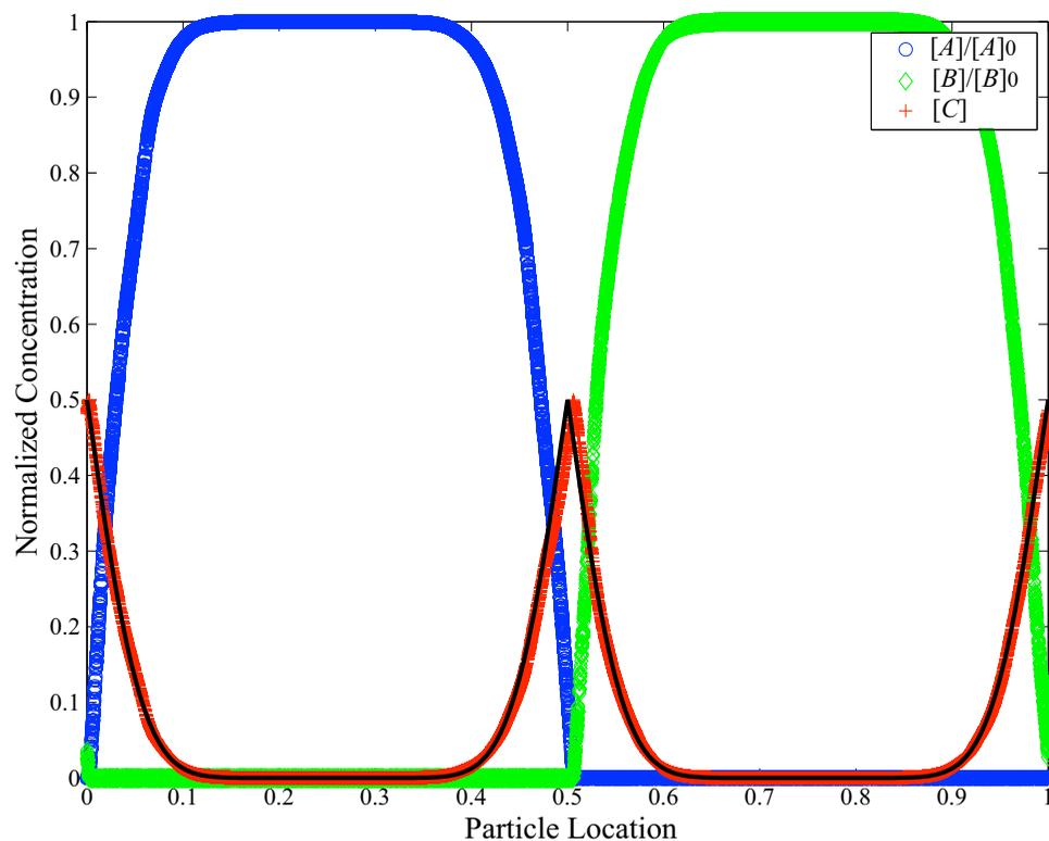
**Figure 6.** Single realization of fast (essentially instantaneous) reaction resulting from initially sharp interfaces between A and B. Periodic domain had initial interfaces at  $x=0=1$  and  $x=0.5$ . Diffusion is simulated purely by mass transfer among fixed-position particles that are uniformly randomly distributed on  $x = [0, 1]$ . Black line is analytic solution.
