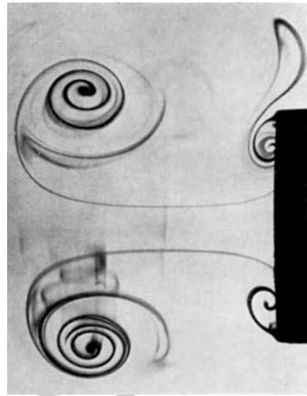
Fig. 5 Formation of a vortex as a cut at a later point of time.
