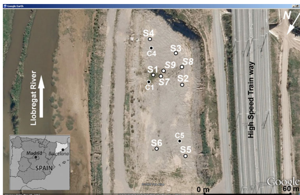
Fig. 1 Satellite image of the Sant Vicenç dels Horts EAP, close to Barcelona (property of Google and ICC, 2007). S-tags refer to the locations of infiltrometer tests; C-tags are excavated pits to observe the local geological stratigraphy
