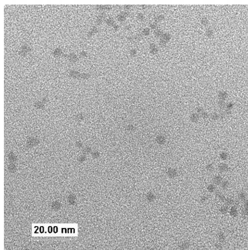
**Figure 1.** Transmission electron micrograph of CdSe/CdS nanoparticles used to prepare the PSS-green QD. The sample was prepared by allowing a solution of nanoparticles in  $\text{CHCl}_3$  to evaporate on a copper-coated TEM grid. The particles exhibit a roughly spherical geometry of 4–5 nm in diameter.
