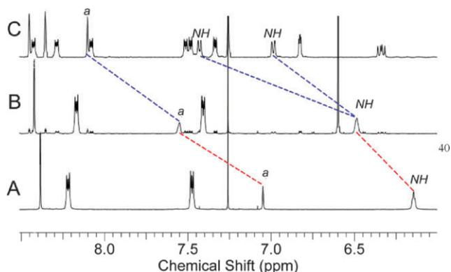
**Fig. 3** Partial <sup>1</sup>H NMR spectra (CDCl<sub>3</sub>) of (A) **1a**, (B) inclusion complex of *N*-ethylmaleimide and **1a**, (C) **2a**.
