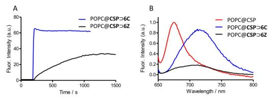
Figure 3. A) Kinetics of association as measured by fluorescence (ex: 685 nm, em: 710 nm). Threading by 6C occurred in seconds while complete threading by 6Z required  $\approx$  20 min. B) Emission spectra (ex: 640 nm) demonstrating POPC@CSP $\supset$ 6Z was partially quenched compared with POPC@CSP $\supset$ 6C.
