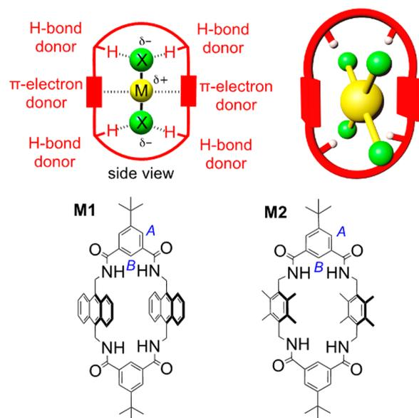
**Figure 1.** (top) Conceptual design of a macrocyclic receptor for square-planar  $\text{MX}_4^{n-}$  anions. (bottom) The two macrocycles used in this study.
