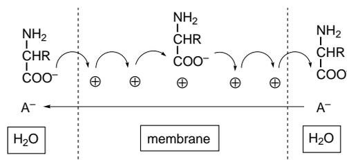
**Fig. 2** A transport process using fixed-site jumping
