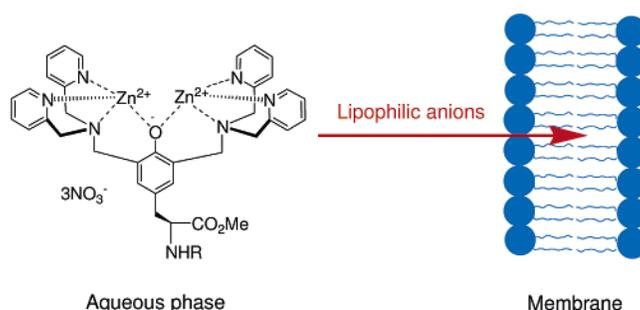
Tyrosine-derived  $Zn^{2+}$  coordination complexes and their fluorescent NBD conjugates are synthesized in a short, high-yielding procedure. The  $Zn^{2+}$  complexes are highly water soluble, but in the presence of sodium laurate they readily transfer into an octanol layer. Furthermore, the NBD-labeled bis- $Zn^{2+}$  complex can partition into vesicle membranes containing anionic phospholipids.
