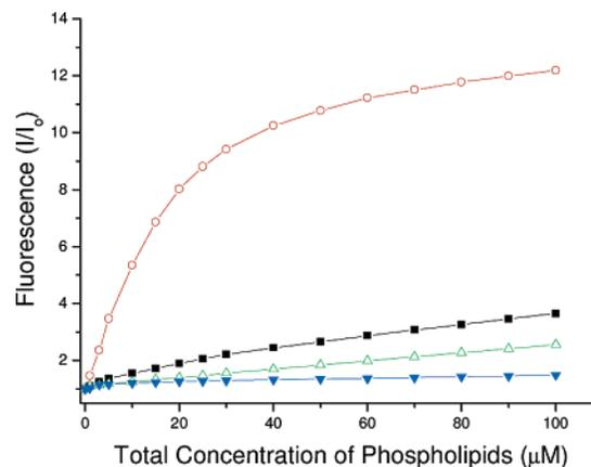
**Figure 5.** Fluorescence titration of **NBD-1•Zn** and **NBD-2•2Zn** ( $1 \mu\text{M}$ ) with vesicles composed of POPC or POPC/POPS 1:1 in buffer (5 mM TES, 145 mM NaCl, pH 7.4). Change in **NBD-2•2Zn** fluorescence upon titration with 1:1 POPC/POPS vesicles (○) or POPC only vesicles (■). Change in **NBD-1•Zn** fluorescence upon titration with 1:1 POPC/POPS vesicles (△) or POPC-only vesicles (▼). The lines in the figure are for clarity; see the Supporting Information for curve-fitting.
