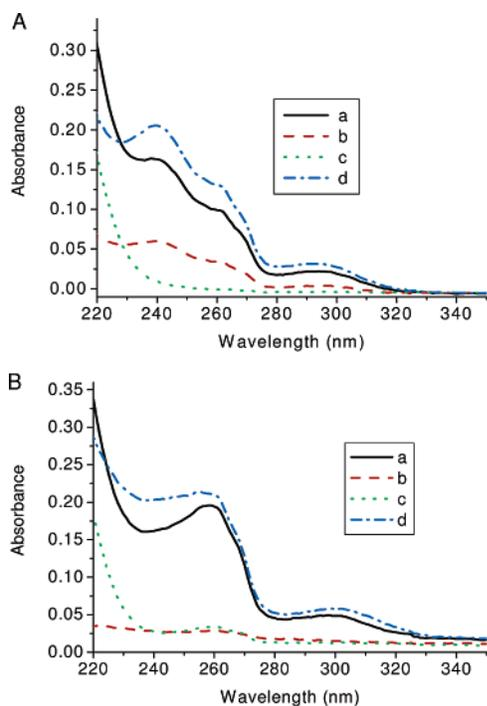
**Figure 2.** UV spectra of (A) **1•Zn** and (B) **2•2Zn** after partitioning between water and octanol in the absence and presence of 1.2 molar equiv of sodium laurate per zinc: (a) aqueous phase without sodium laurate; (b) organic phase without sodium laurate; (c) aqueous phase with sodium laurate; (d) organic phase with sodium laurate.
