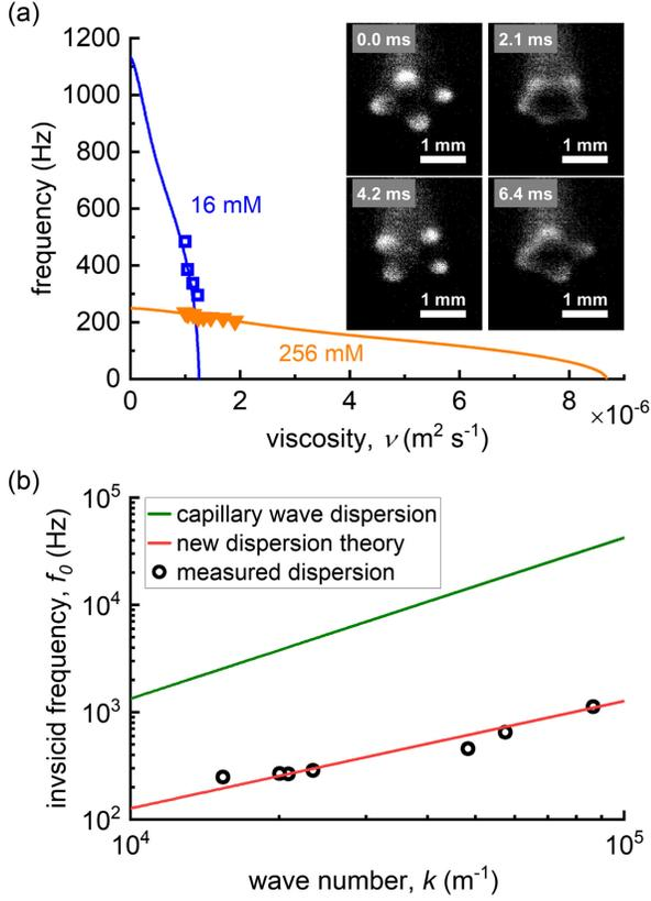
FIG. 2. (a) Pattern oscillation frequencies measured using high-speed imaging (inset) for various solution viscosities and ionic strengths. (b) The inviscid frequency  $f_0$  for  $\nu = 0$  and wave number  $k$  were extrapolated using Eq. (4) for various values of ionic strength. Extrapolated inviscid frequencies are compared to the traditional capillary wave dispersion and Eq. (5).
