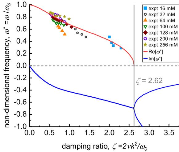
FIG. 4. The physical roots of Eq. (6) as a function of  $\zeta$  consist of a frequency component,  $\text{Re}[\omega^*]$  plotted in red, and a damping rate,  $\text{Im}[\omega^*]$  plotted in blue. Nondimensionalized frequency data, for various values of solution viscosity and ionic strength, collapse onto the real part of the root of Eq. (6).
