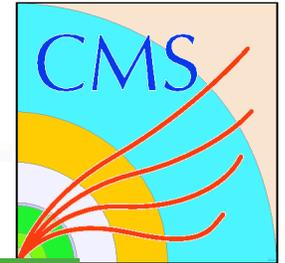
H $\rightarrow\gamma\gamma$  photons: Barrel 20-50 GeV
