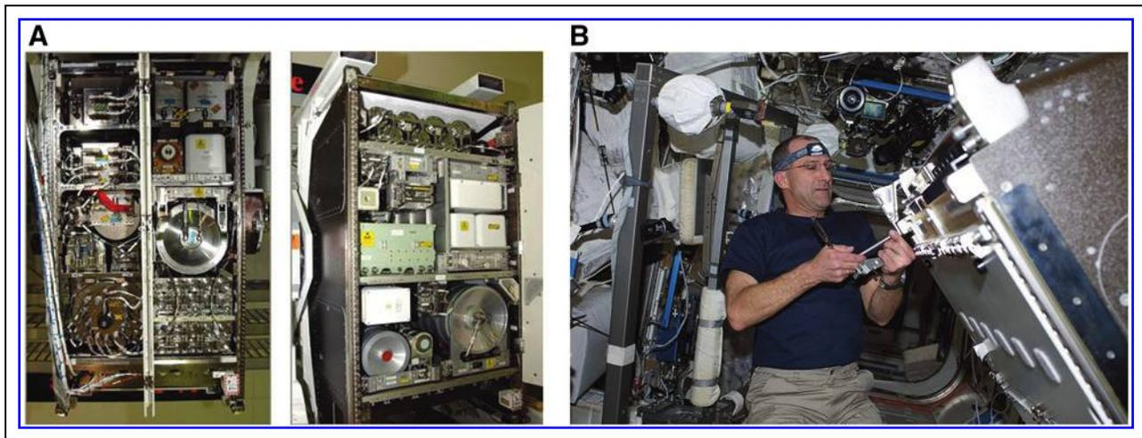
**FIG. 3. (A)** The ISS water recovery component of the Environmental Control and Life Support System (NASA). **(B)** NASA astronaut Don Petit installs the WRS into the Destiny Laboratory on the ISS in November 2008. Image Credit: NASA.
