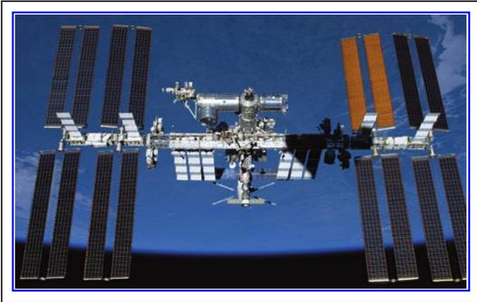
**FIG. 1.** Orbiting by Earth’s horizon and the blackness of space, the International Space Station (ISS) is 357 feet (109 m) end-to-end and almost spans the 360-foot area of an American football field, including the end zones. With 33,023 cubic feet of pressurized volume, the space station now has more livable room than a conventional 5-bedroom house. Image Credit: NASA.
