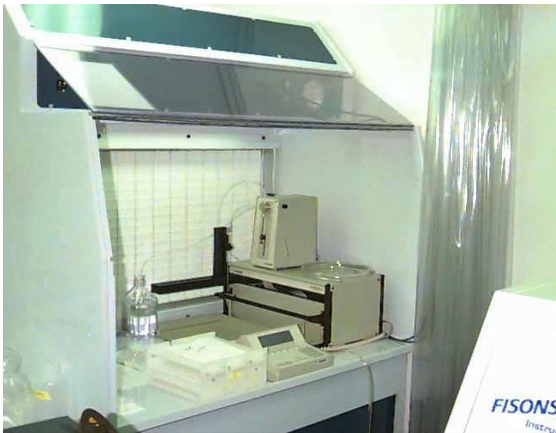
FIGURE 2: PolyDesign HEPA-filtered Laminar Flow Work Bench
