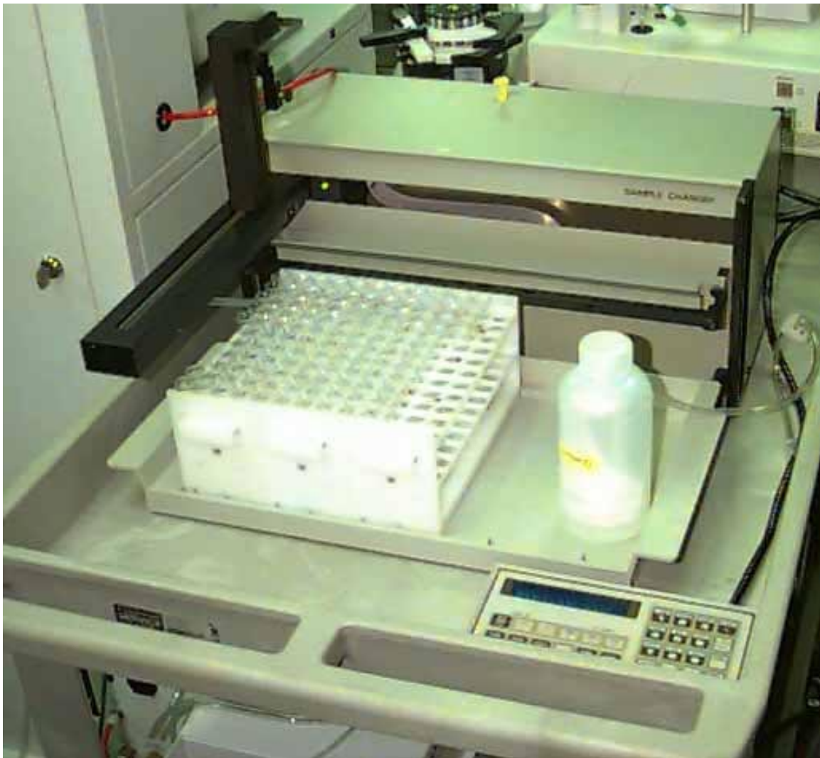
FIGURE 10: The Gilson Autosampler which allows automated runs of up to 150 samples with a wash procedure in-between each individual sample tube.
