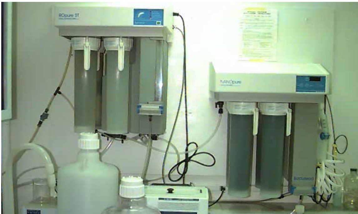
FIGURE 3: The Barnstead-Thermolyne 18 Mega-Ohm Ultrapure Water System
