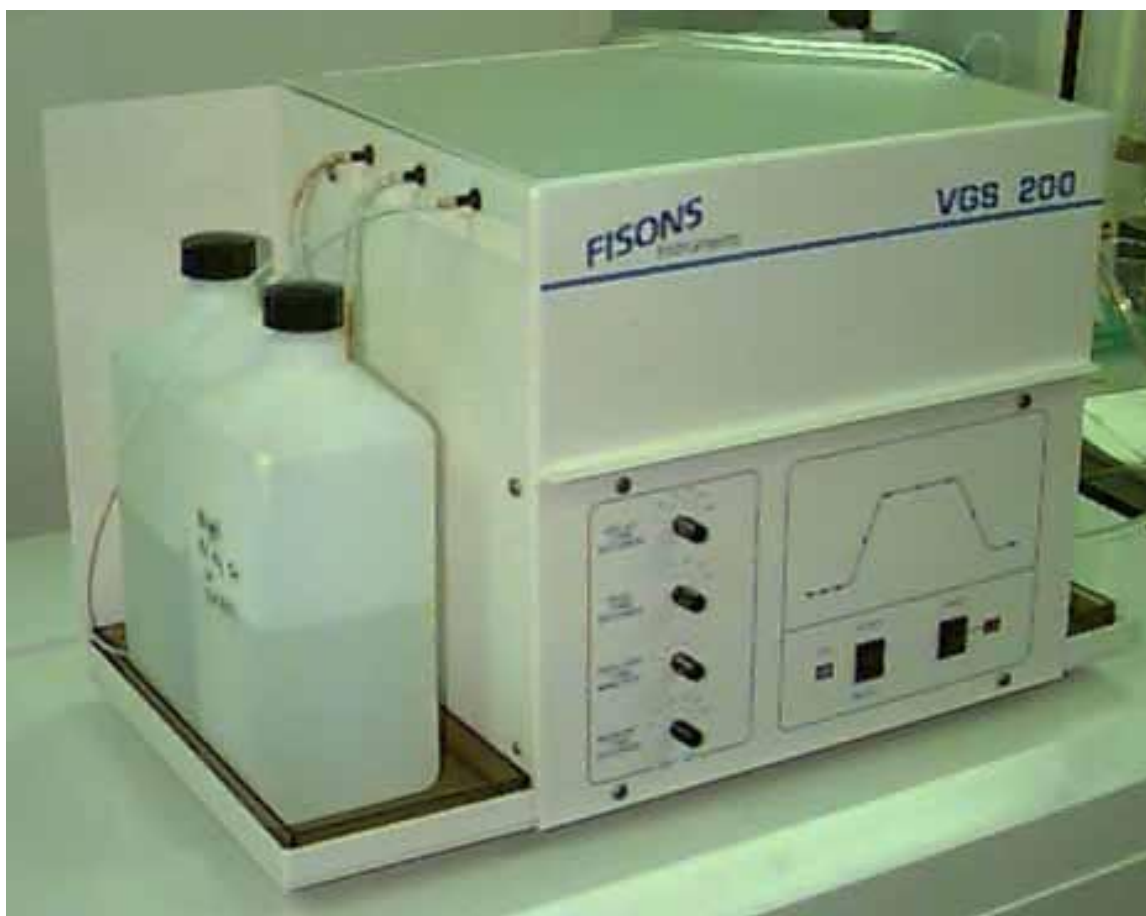
FIGURE 7: The FISIONS VGS 200 Hydride Generator for analysis of elements which form gaseous hydrides at ambient temperatures (i.e., As, Bi, Ge, Pb, Sb, Se, Sn, & Te), as well as elemental Hg.
