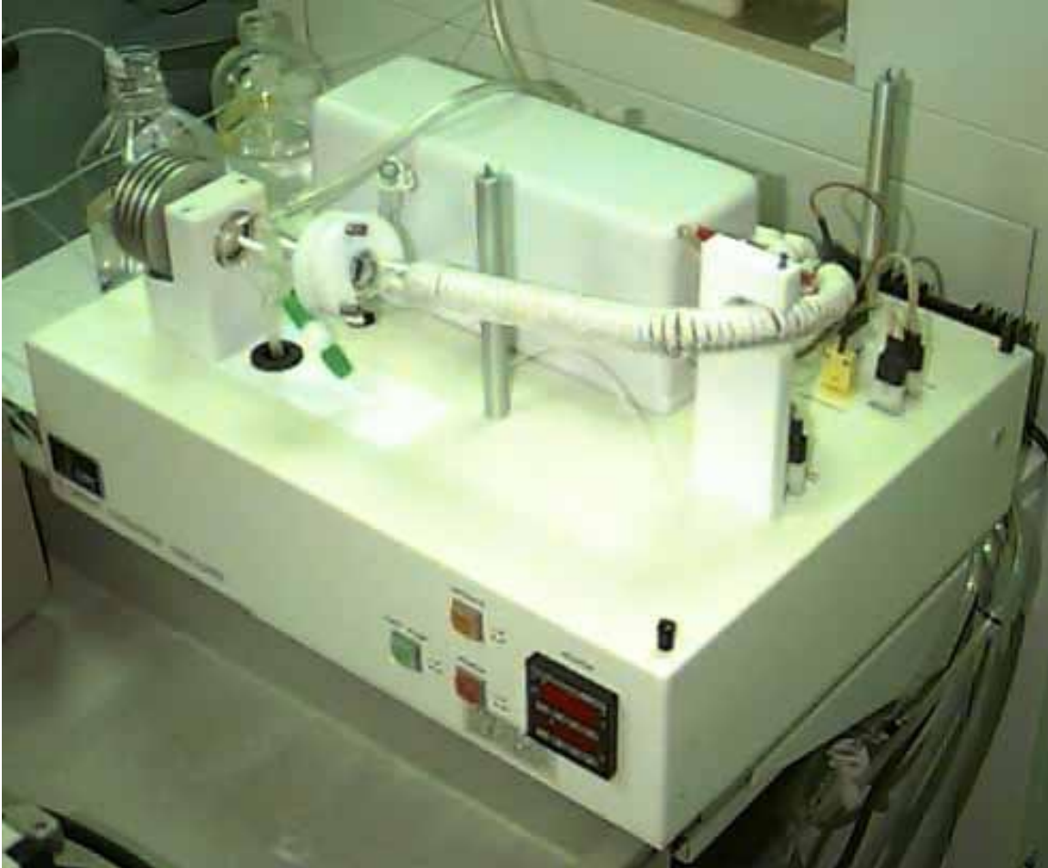
FIGURE 6: The CETAC Ultrasonic Nebulizer for ultra-trace element analysis (pico-gram/gram detection).
