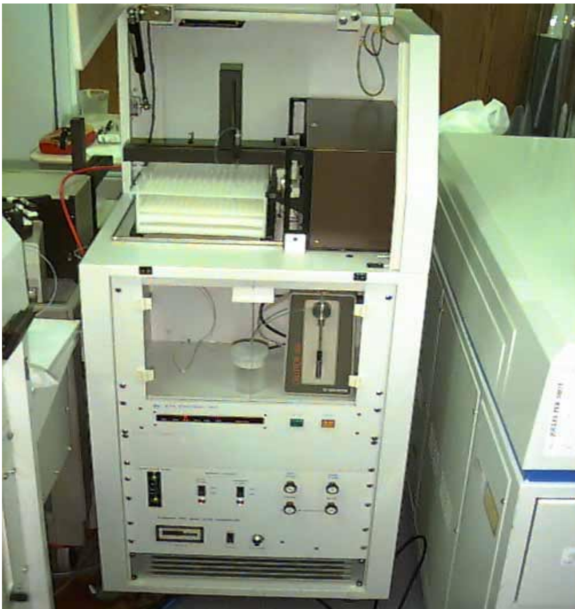
FIGURE 8: The Mark IIIa Electrothermal Vaporization Unit for the ultra-trace element analysis of micro-liter samples.
