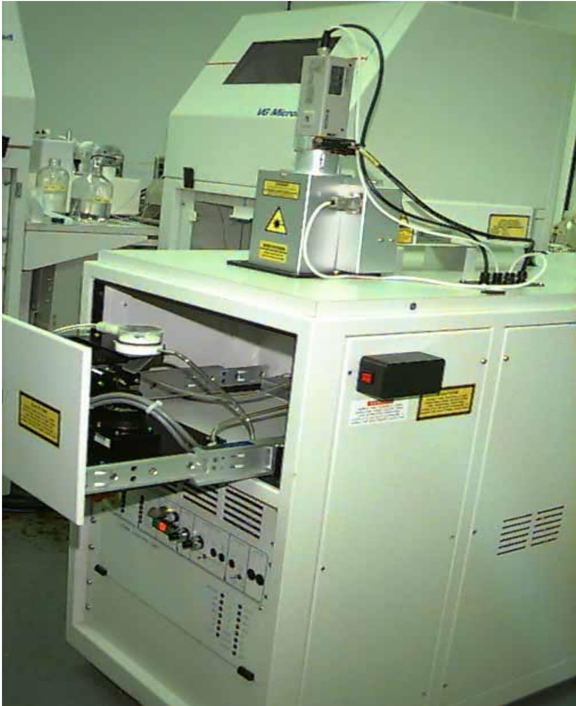
FIGURE 5: The Laser Ablation Microprobe now capable of generating three wavelengths of laser radiation: 1064 nm (IR), 532 nm (visible), 266 nm (UV). This allows micro-sampling of solid samples including petrographic thin sections.
