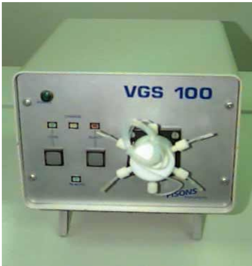
FIGURE 9: The VGS 100 Flow Injector for use in analyzing samples containing high total dissolved solids (e.g., seawater, brines, etc.).
