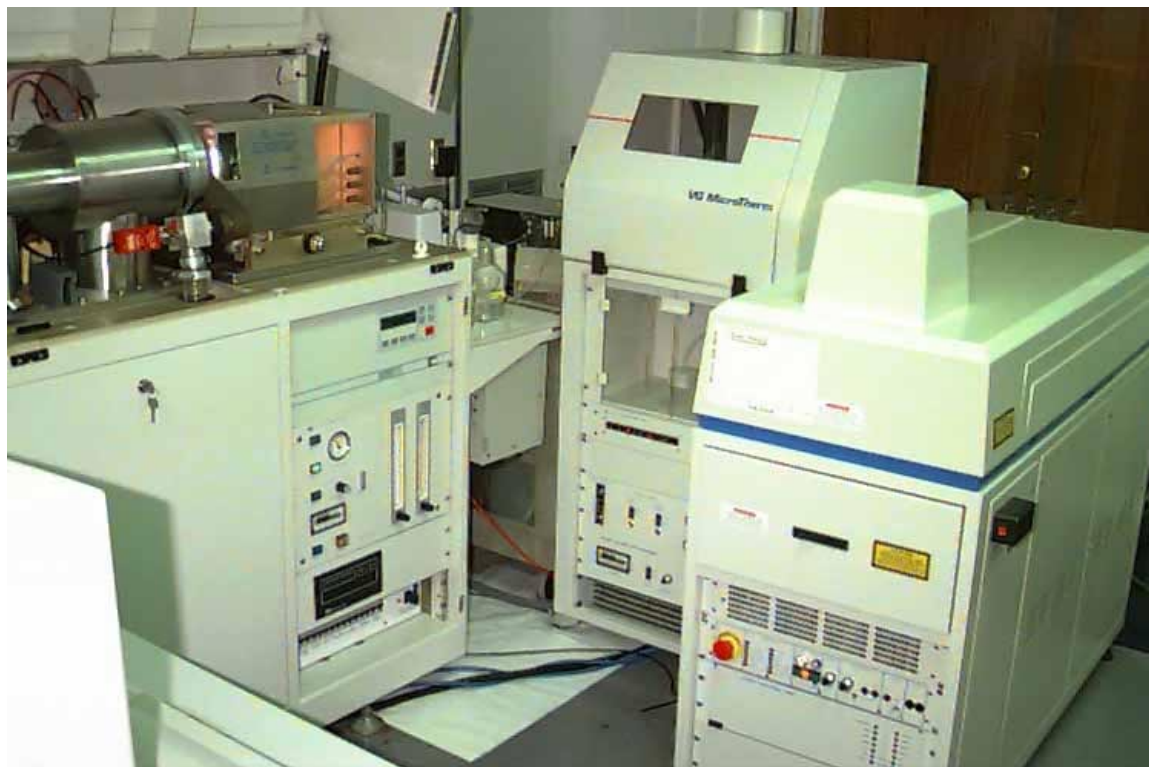
FIGURE 1: View of the ICP-MS Laboratory showing the PQII STE ICP-MS, Electrothermal Vaporization, and Laser Ablation units
