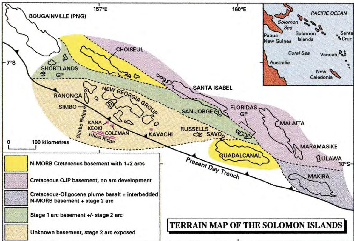
Fig. 2. Terrain model of Solomon Islands. Five crustal units are identified on the basis of distinctive lithology, age, and geochemistry of basement sequences and presence/absence of arc sequences. See text for details.
