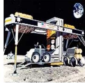
Concept of remotely driven surface vehicles mine and transport lunar soil to the plant, where the oxygen is extracted, liquefied, and pumped into waiting storage tanks. (Image: NASA/JSC)
