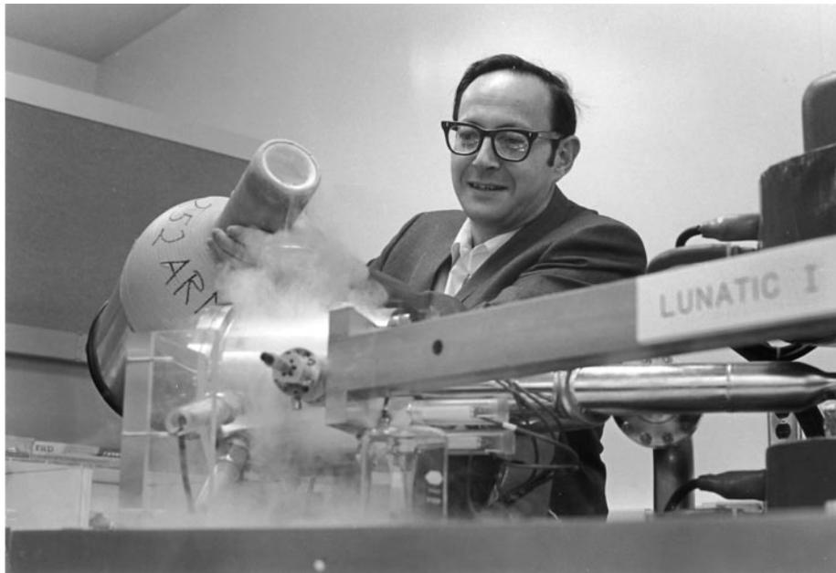
**Figure 2** Filling liquid nitrogen in the ion source trap of the Lunatic I (circa 1970). Caltech archives.
