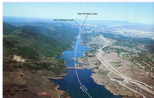
Box 15.3 — FIGURE 2 Part of the San Andreas fault. View northward toward San Francisco. Lakes occupy the fault zone. Hills to the left of the fault are moving northward.
