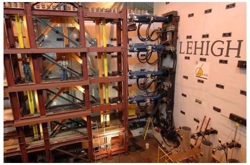
Innovative earthquake-resistant self-centering (SC) steel frame systems are being developed to be damage-free and without residual drift under the design basis earthquake (DBE). This presentation summarizes hybrid earthquake simulations on large-scale 4-story SC steel frames at the Lehigh NEES equipment site that are being used to validate performance-based design procedures for these SC steel frame systems.
