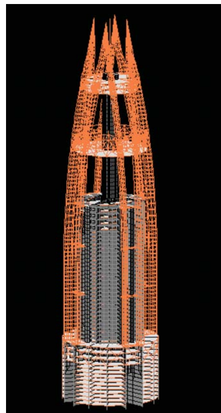
Figure 11. Finite Element Model of Spire and Crown
