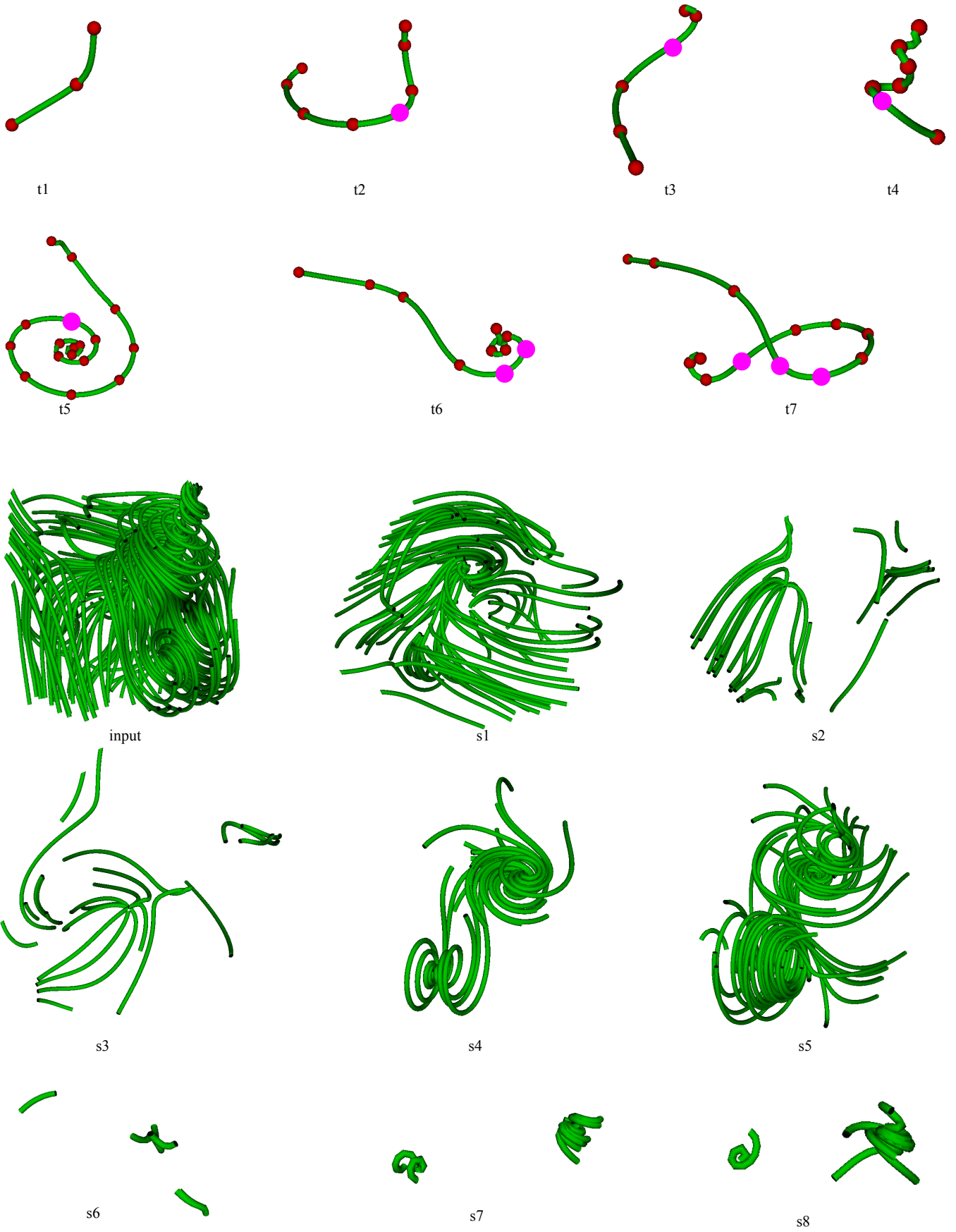
Figure 10: Seven streamlines of the five critical points data set were manually segmented ( t_1 - t_5 ) to train the classifier. Eight ( s_1 - s_8 ) clusters of streamline segments were generated.
