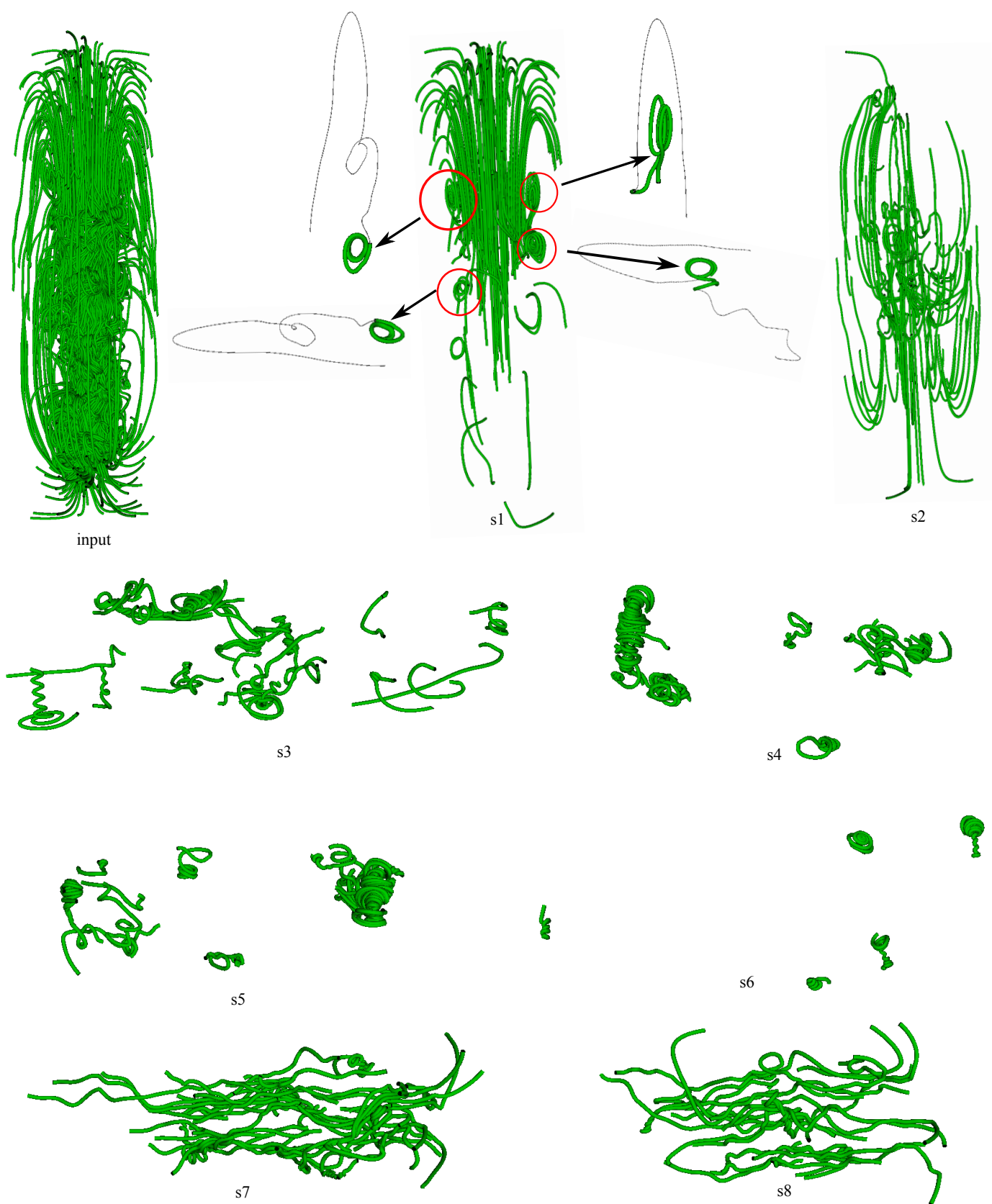
Figure 11 (cont.): Eight ( s_1 - s_8 ) out of 14 clusters of streamline segments of the solar plume data set are shown here. Notice how the interesting features such as spirals and turbulent features are successfully extracted.
