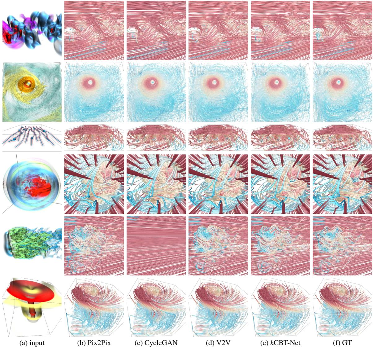
Figure 8: Streamline visualization results with different methods. Top to bottom: streamlines traced from translated vector fields with half-cylinder (VM (640)), hurricane (VM), supercurrent (RHO), supernova (VM), Tangaroa (VM), and tornado (VM) input scalar fields.
