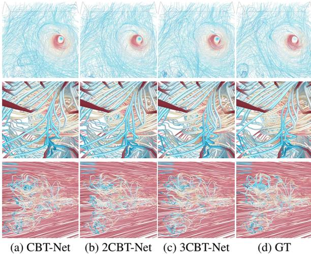
Figure 1: Streamline visualization results with different  $k$  for  $k$ CBT-Net. Top to bottom: streamlines traced from translated vector fields with hurricane (QVAPOR), supernova (VM), and Tangarao (VM) input scalar fields.
