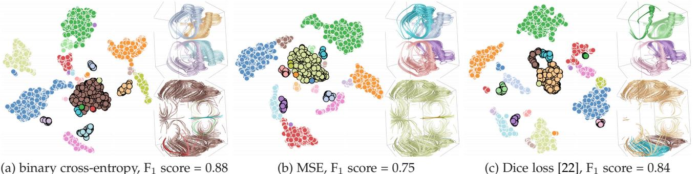
Fig. 5: Comparison of feature descriptors under different loss functions using the two swirls data set. All generate 25 clusters through DBSCAN. The selected streamline clusters are highlighted and shown in the t-SNE view.
