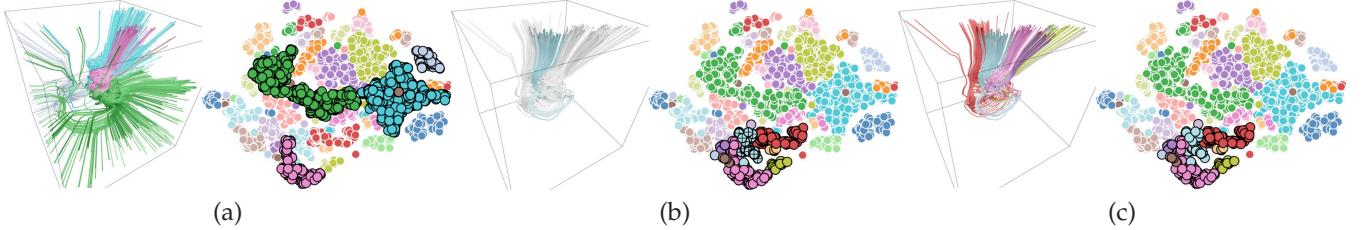
Fig. 2: A sequence of cluster interactions in the t-SNE view and the linked volume view using the supernova data set: (a) choosing multiple clusters simultaneously, (b) expanding from one selected cluster highlighted at the bottom of the t-SNE view in (a) to its neighboring clusters, and (c) looping through each of these clusters (the focal cluster is highlighted with additional + signs). In (c), the remaining streamlines in the neighborhood are drawn in gray as the context.
